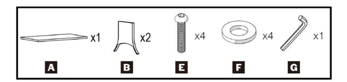
Loosely secure the upper table base ( $\mathbf{B}$ ) to the table top ( $\mathbf{A}$ ) using M6 x 35mm screws (E), washers (F) and the allen key (G). Once secure tighten all the bolts.
