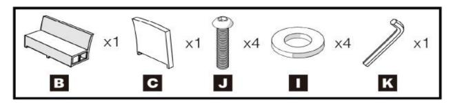
Position the arm (C), onto the armless sofa (B). Loosely secure using M6 x 35mm screws (J), washers (I) and the allen key (K). Tighten when all bolts are fitted.
